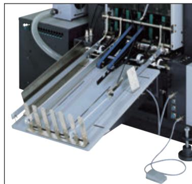
This tray was designed specifically to handle difficult-to-align papers such as NCR paper, or those sheets with spot carbon. In order to assure a perfectly aligned stack of collated sets, the jogger, run by an independent motor, vibrates the sets into place. The tray also descends automatically as it receives the collated sets. To reset the jogger receiving tray and continue operation, simply push the foot pedal.
