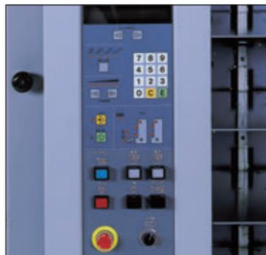
Horizon's highly advanced sensor and electronic controls make for adjustment-free, easy operation. Presetting of the number of completed sets per grouping, the total count, as well as placement of the front and back covers allows for flexibility or programming. State-of-the-art sensors detect such errors as miss or double sheet feeding, incorrectly aligned sheets, as well as imperfect sheets.
